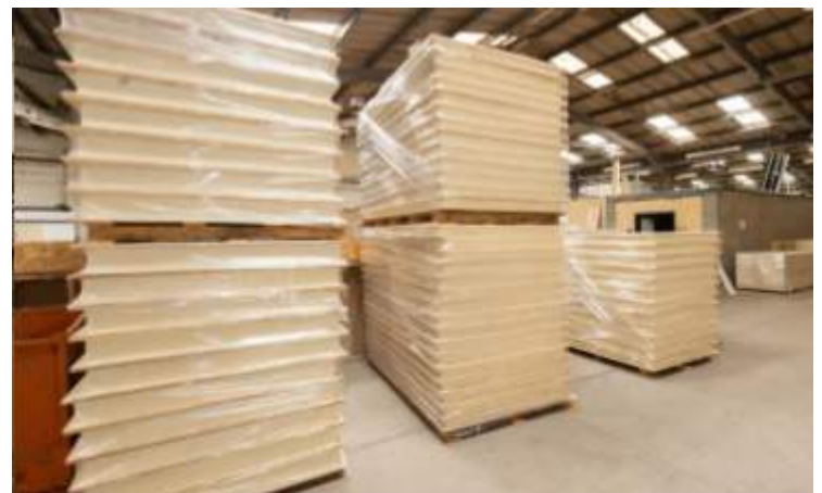
Finished SIP Panels
